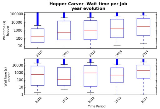
Figure 11: Jobs' wait time evolution for each workload year. Trend: All systems increase wait time. Carver lower wait time in 2011.
